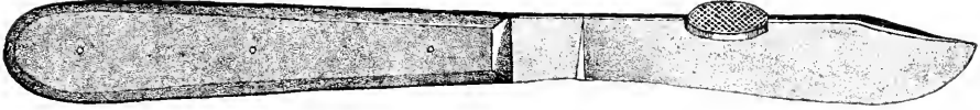
FIG. 15.—Cartilage-knife with projection on back upon which the index-finger rests when making incisions. (Two-thirds natural size.)
